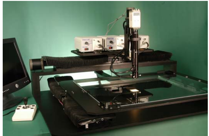
Open-frame half-gantry configuration with back illumination
